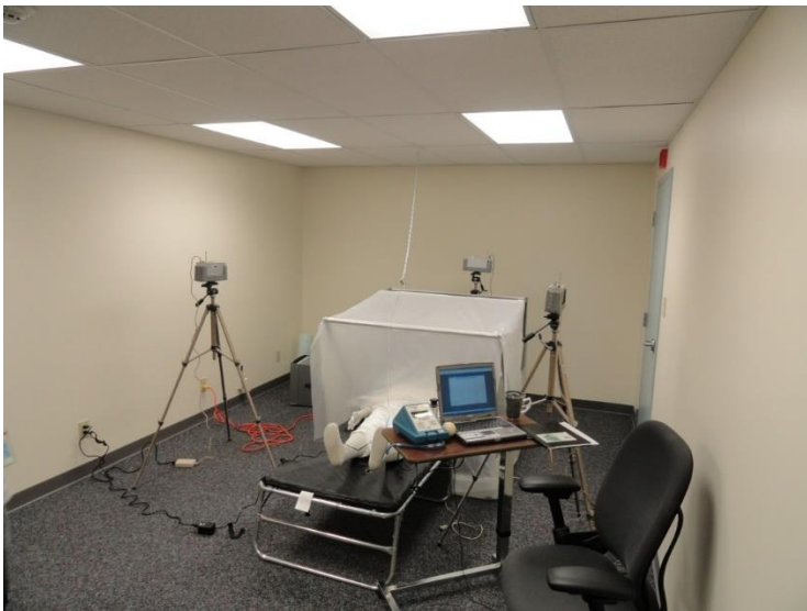
CDC/NIOSH Photo Showing Ventilated Headboard Tested In Reverse Isolation Mode:
