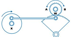
While wheel **X** turns round and round in the direction shown, wheel **W** turns
